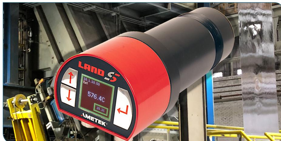
Non-contact temperature instruments measure the infrared radiation from the object, which depends on that object's temperature and emissivity, and possible reflection from other objects such as furnace walls or heat sources. The object's emissivity is mainly dependant on the material, the surface condition and the viewing angle.
