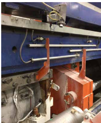
SPOT AL EQS and Actuator scanning a profile along the billet as it arrives at the press
