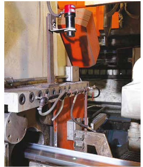
SPOT AL EQS on a manually adjusted mounting at the press exit.
