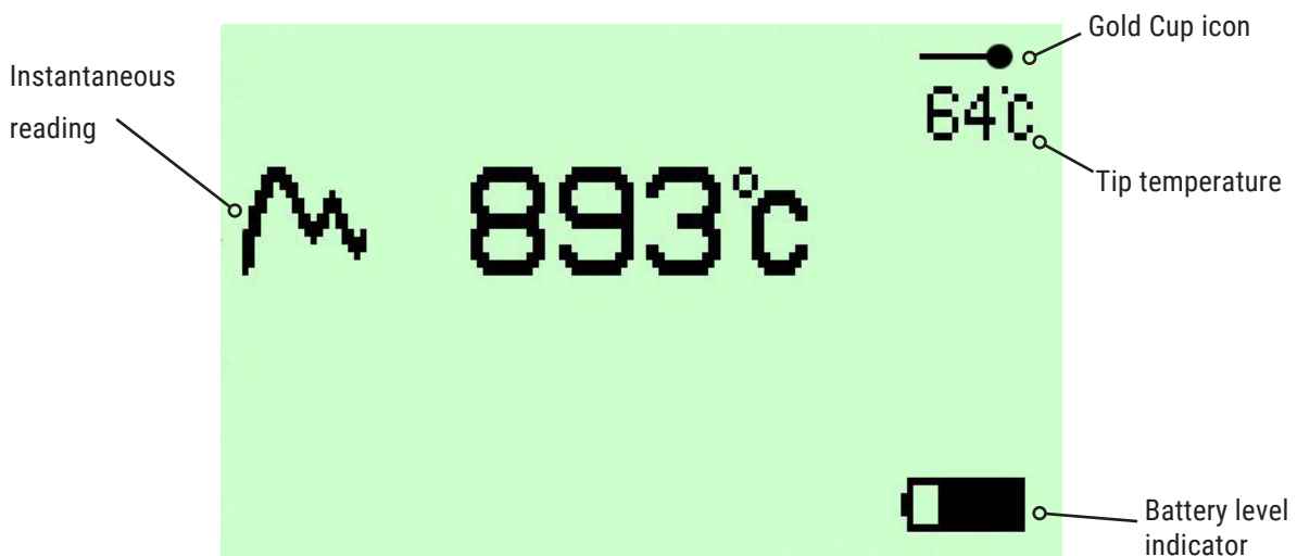
Fig. 7-1 Typical Measure Mode display
