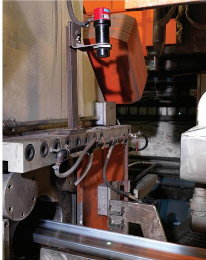
on the pyrometer or remotely using the integrated webserver via TCP/IP with a standard web browser, the pyrometer measures an accurate product temperature for approximately 90% of all aluminium alloys, without the need for additional adjustments.
