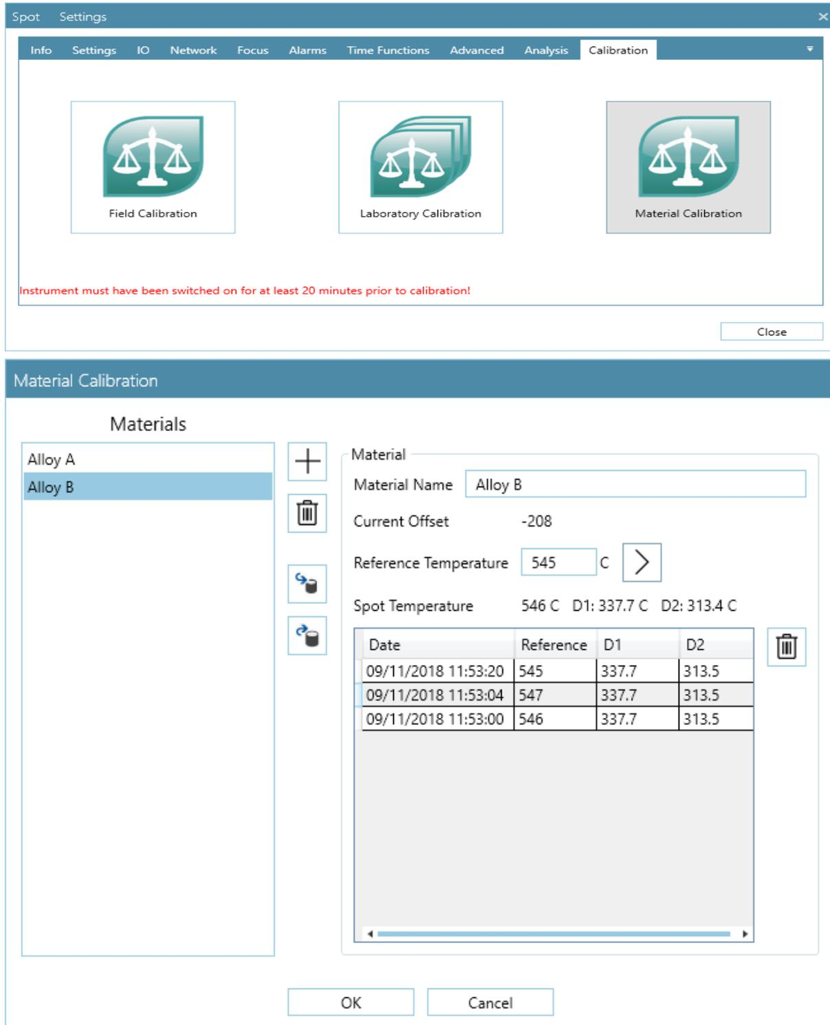
The screenshot shows the 'Spot Settings' window with the 'Calibration' tab selected. Three calibration options are visible: Field Calibration, Laboratory Calibration, and Material Calibration. A red warning message states: "Instrument must have been switched on for at least 20 minutes prior to calibration!".
