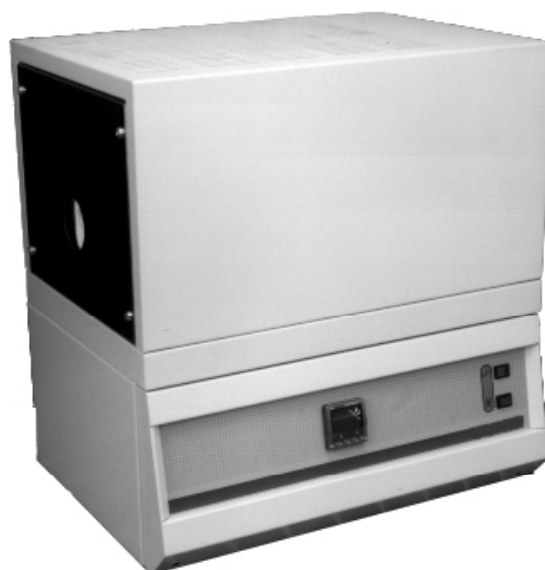
Fig. 1 Landcal black body calibration source type R1500T
