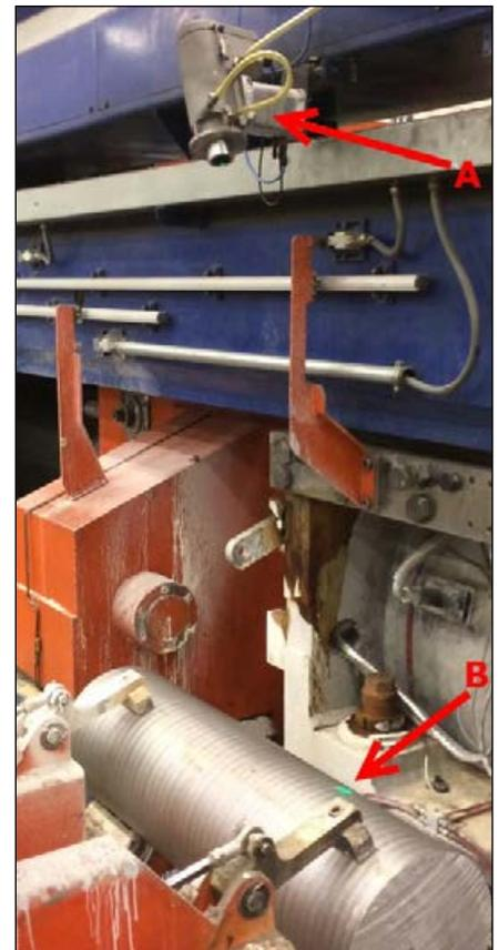
Figure 2. A pyrometer with a motorized actuator (A) scans the temperature of the billet length using a targeting LED spot (B).
