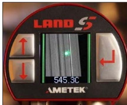
Figure 1. The pyrometer provides video sighting to ensure precise alignment.
