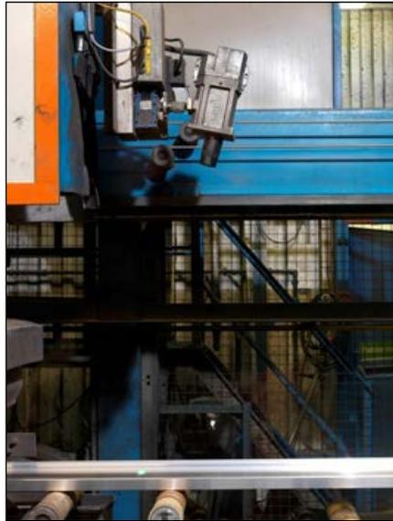
Figure 4. A SPOT AL EQS being implemented at the exit of the quench.
