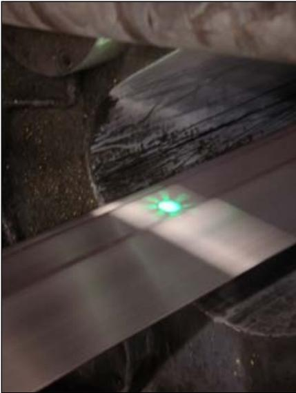
Figure 3. At the press exit, the pyrometer targets an extruded profile by emitting a green LED spot to improve the accuracy of the temperature measurement.
