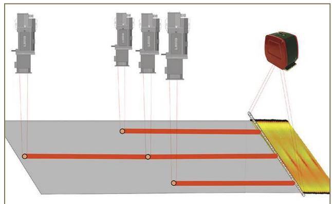
**Fig. 4.** Comparing a single pyrometer, three pyrometers and a scanner
