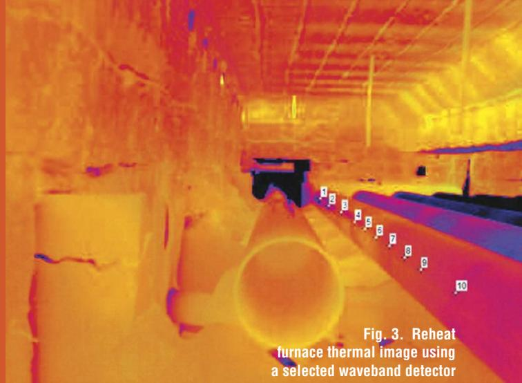
Fig. 3. Reheat furnace thermal image using a selected waveband detector
