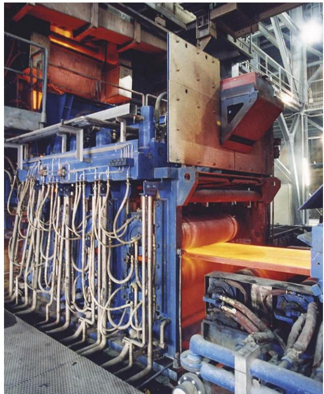
**Fig. 5.** A scanner is mounted at a continuous caster exit, after the straightener, just before the slab is cut. The red water-cooled protective enclosure houses the scanner and is mounted above an angled heat-deflecting plate.
