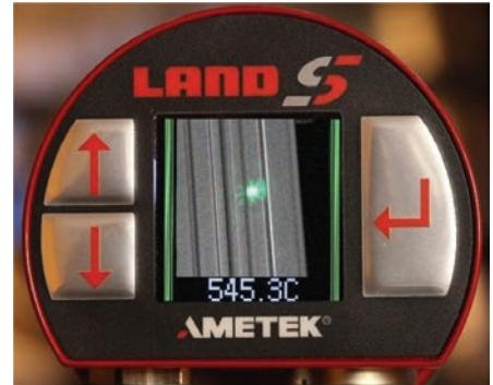
Fig. 4. Pyrometer image view of the target with LED illuminated
