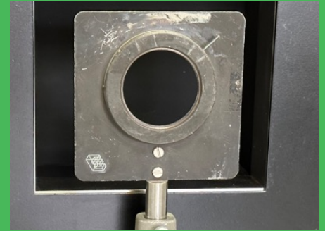
A test was performed with multiple high-temperature targets (a heated metal target at a temperature of around 150 degrees Celsius in front of a hot plate at around 440 degrees Celsius).
