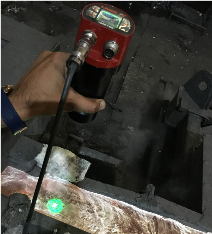
The SPOT's pulsed LED sighting pattern ensures optimum focus
