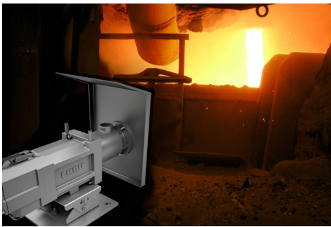
SDS V2 imager with heavy industrial enclosure
