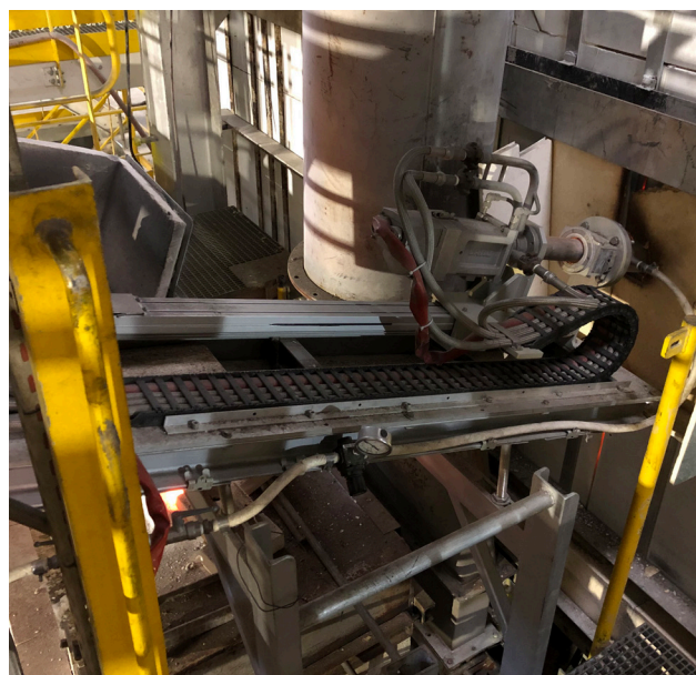
NIR-B Glass inserted through the furnace wall
